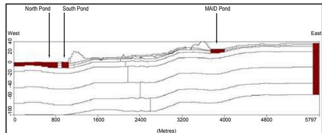
Figure 8. Cross-section of Specified Head Boundary conditions
