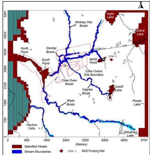
Figure 7. Plan view of Specified Head Boundary conditions
