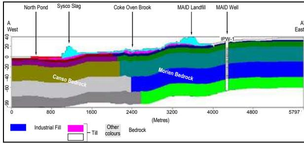
Figure 3. Domain cross-section (see Figure 4 for location)
