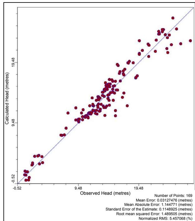
**Figure 9.** Calculated versus Observed Hydraulic Heads
